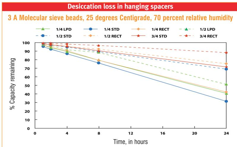
The graphic above shows desiccation losses by type of spacers and their dimensions, in inches. It features data on low-profile designs, rectangular and standard box spacers.
